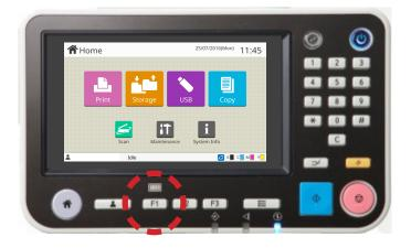
A] Press the > F1 button > on FW Operation
