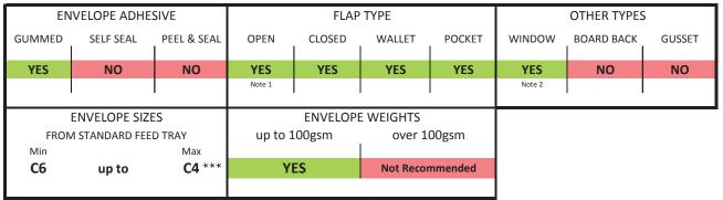
Note 1: Open flap Self Seal are not considered suitable as the adhesive can transfer onto machine parts
